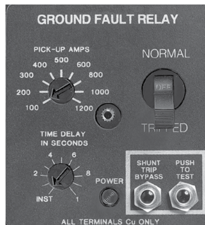
Ground Fault Relay
